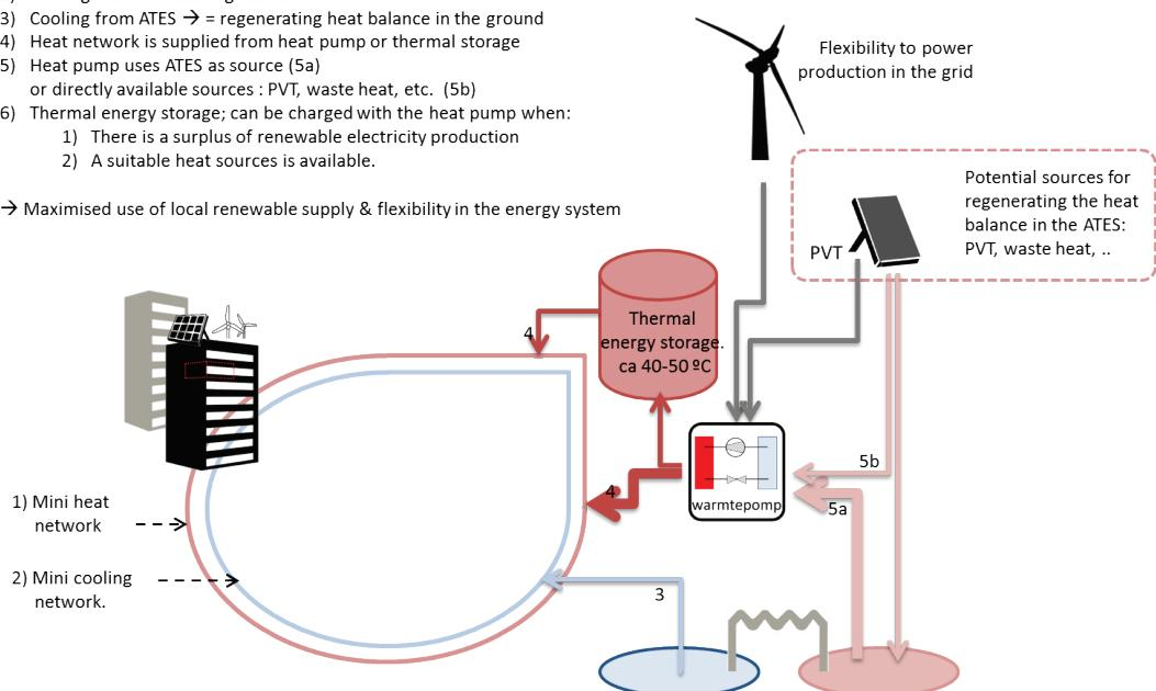
Figure 5. Scheme of a fourth energy concept for the new buildings developed to overcome the shortcomings of the basic variants 1, 2, and 3.
